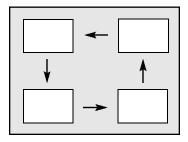
**Note:** Each press of the MovE button will shift the PIP window one position.
